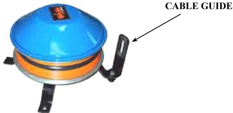
A cable guide must also be installed at the end of each boom section to keep the cable in straight line. Sagging of the wire would cause non-linearity of the length measurement.
