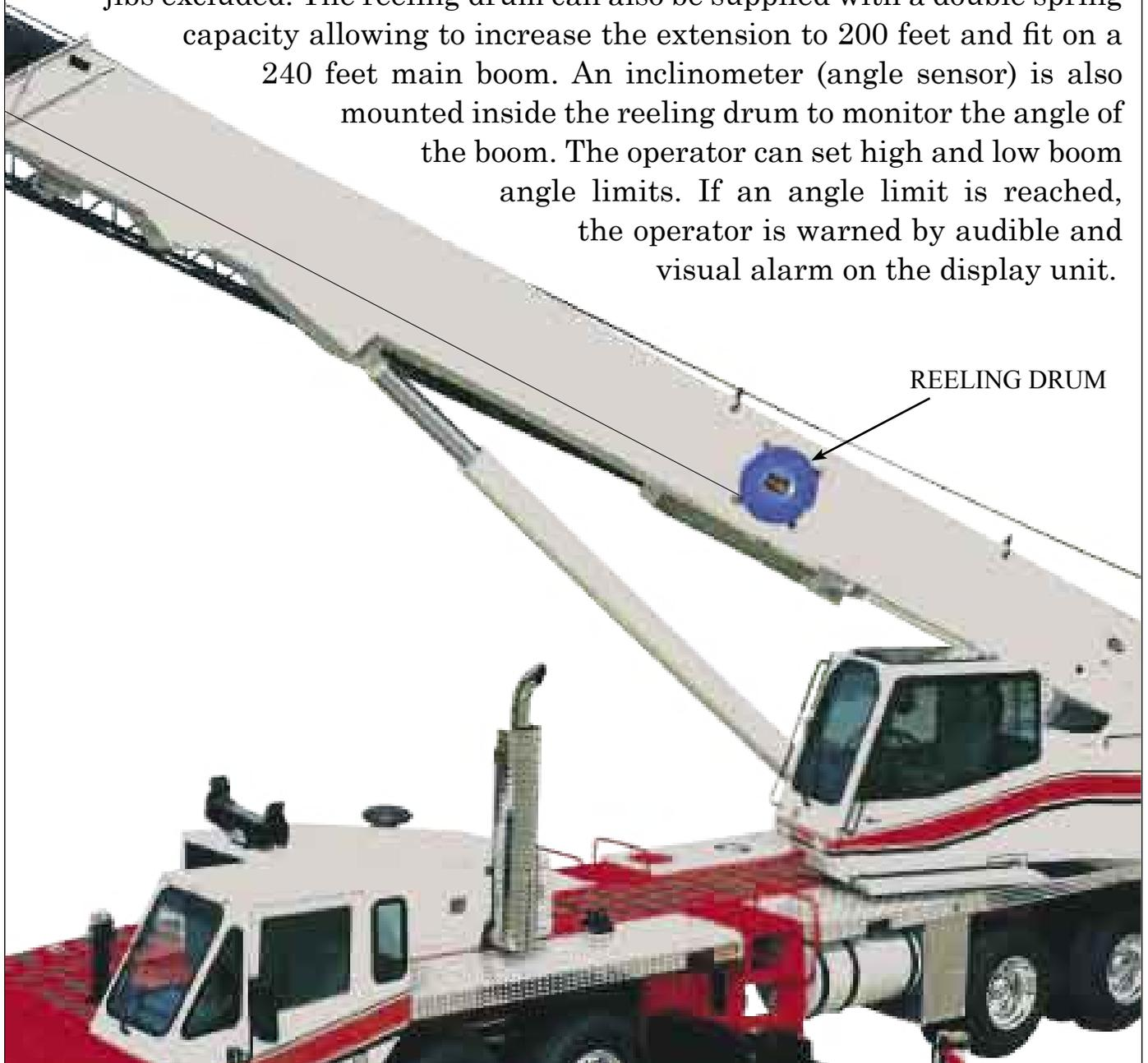
The reeling drum must never stick above or below the boom as this would increase its vulnerability to collide with objects. It should be located equally distant from all chords and ribs to prevent stresses when welding lugs.
