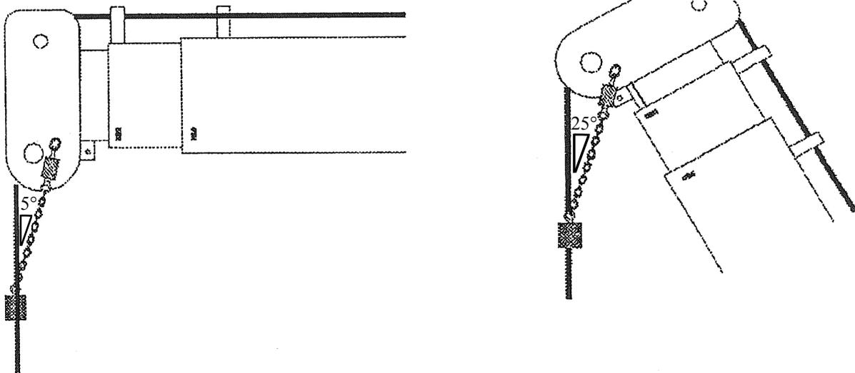
Once the mounting location is determined, weld the mounting plate in the proper position. The weight will be clamped around the proper hoist rope then attached to the bottom of the switch. Please note that the anti two-block weight should move freely on the hoist rope and not bind on the hoist rope. If the weight is too tight on the hoist rope, false two-block indications will occur.
