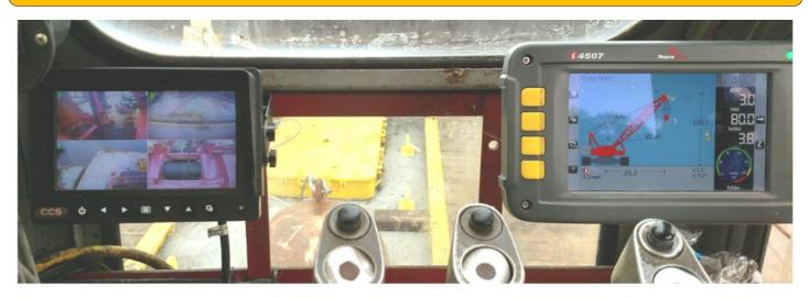
Shown on the crane dash with the CCS4 camera monitor to left and Rayco/Wylie i4507 LMI to right
