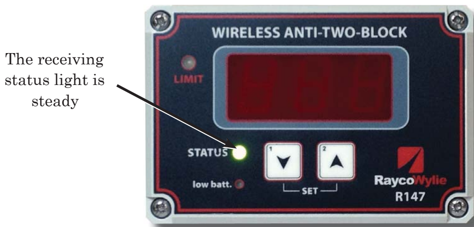
Fig. 4: R147 Normal Mode of operation (no two-block)
