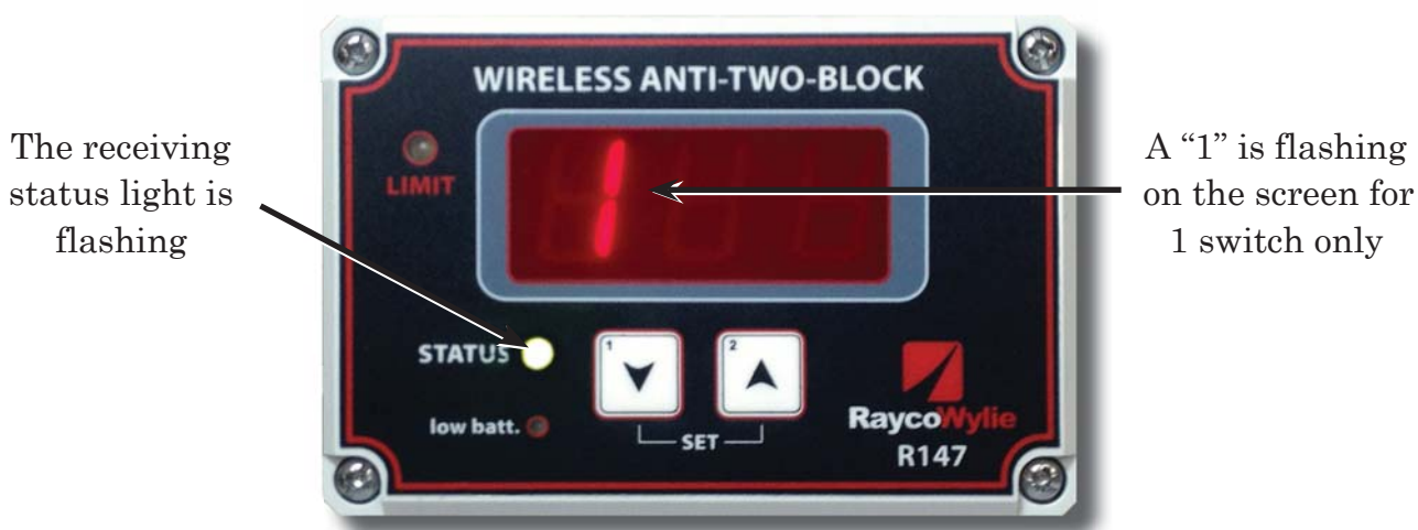
Fig. 3: R147 Waiting for transmission from the ATB switch
