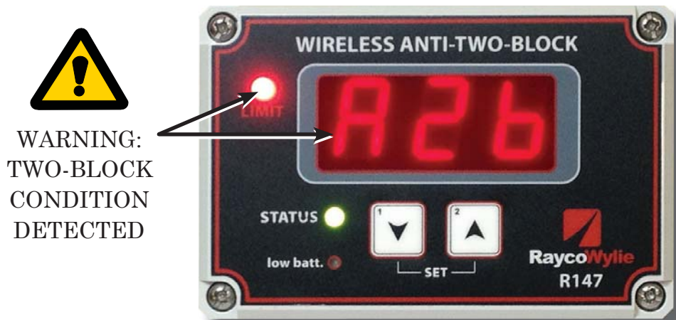
Fig. 5: R147 in a Two-Block condition
