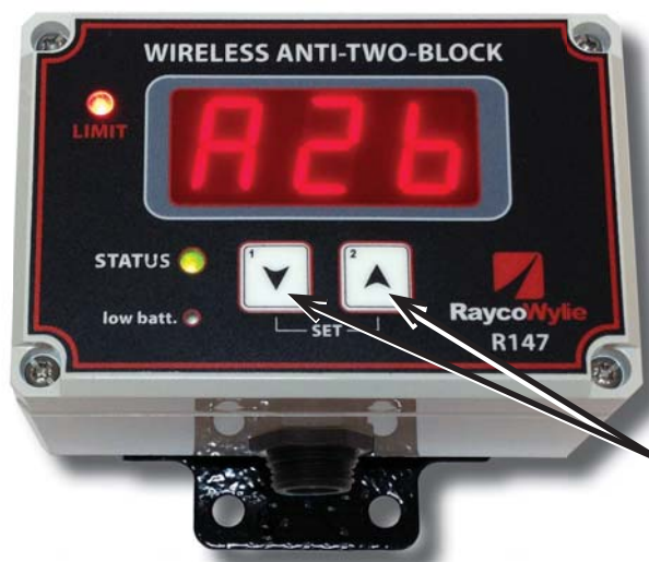
Fig. 6: Bypassing the R147 system
