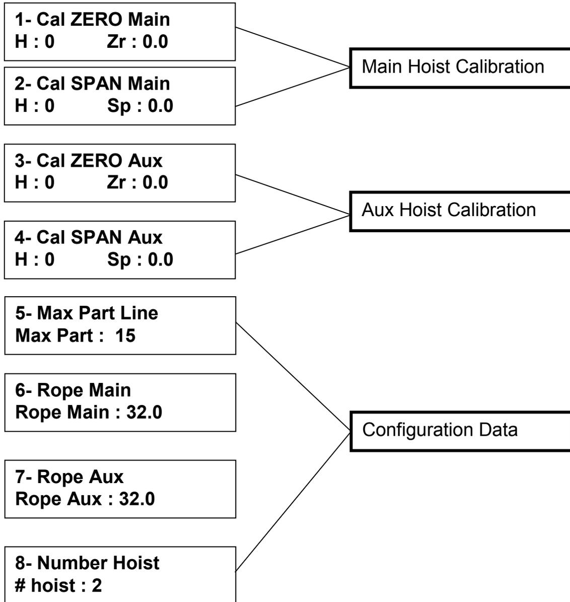
System with load and angle sensor option sequence numbered 1 to 10:
