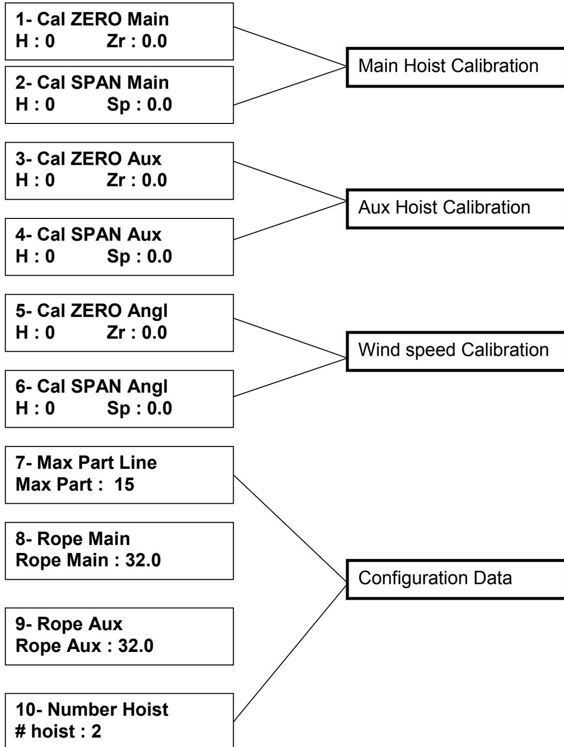
To enter into the calibration mode, unscrew the top cover to have access to the internal circuit. Turn the system on; wait until the system loads the basic screen display with load. Remove the "CAL" jumper located on the I/O Board. The system will alarm using the ATB light and buzzer. Press the push button located on the CPU Board.
