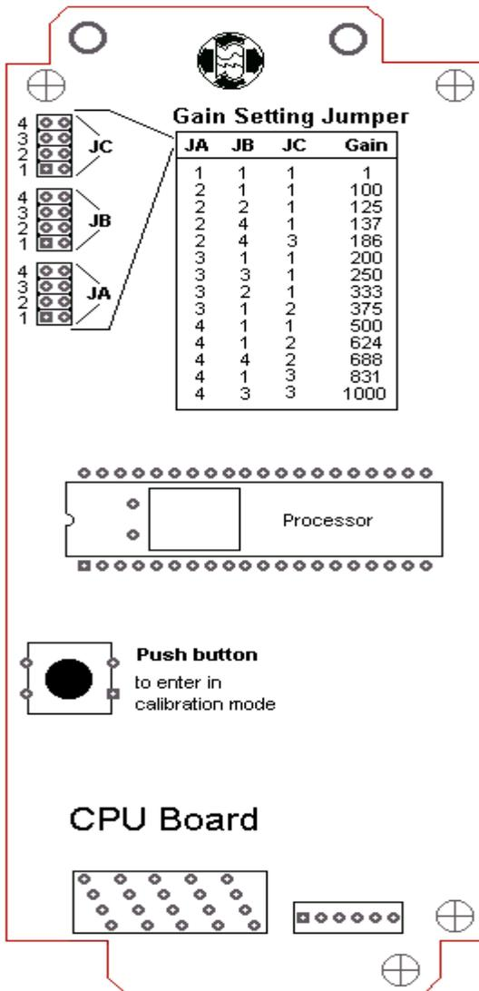
The gain setting is located on this board. Use 3 small jumpers to configure it. Default value is 333.
