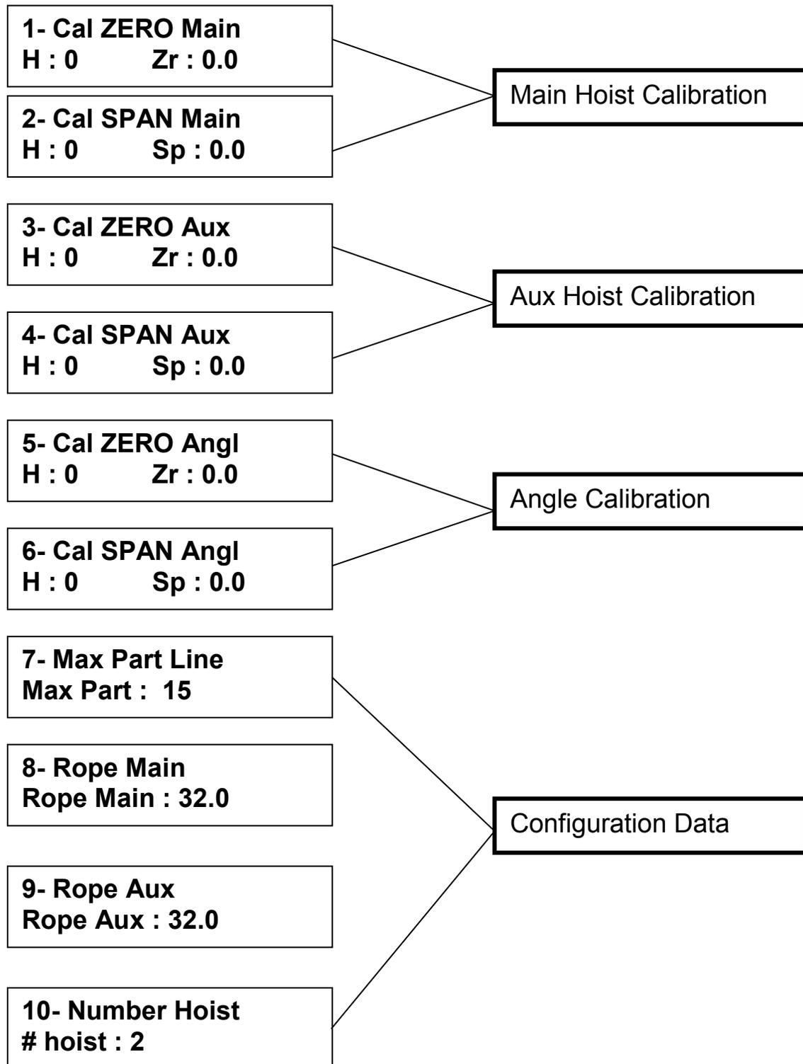
System with load and length sensor option sequence numbered 1 to 10:
