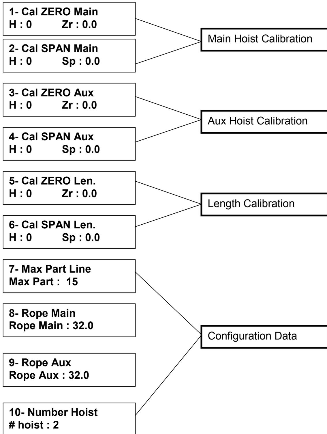
System with load and wind speed sensor option sequence numbered 1 to 10:
