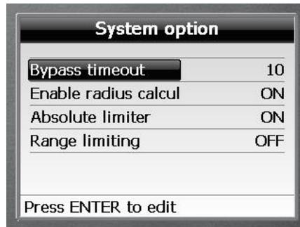
**Bypass Timeout.** Time allowed in seconds before to re-activate the motion cut after pressed the Bypass key in normal mode.
