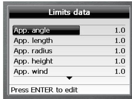
Set the approach gap for each limit in turn, angle approach gaps are in degrees, length, radius and height gaps are set using the calibration units.
