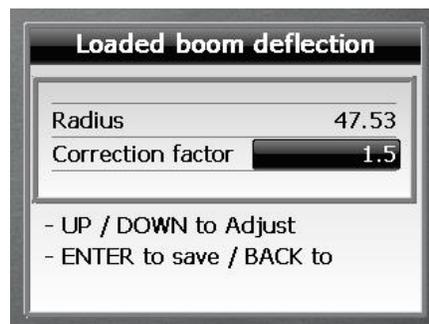
Carefully lift the test load until it is just clear of the ground. Accurately measure the actual radius of the suspended load from the centre line of slew of the machine.
