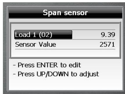
To span the load sensor, position the boom at the same safe radius for the large test load as above and slowly lift the large test load until it is just clear of the ground.
