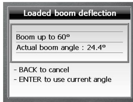
Adjust the boom angle to the target angle, when the boom is at the correct angle for calibration the display will change to show:
